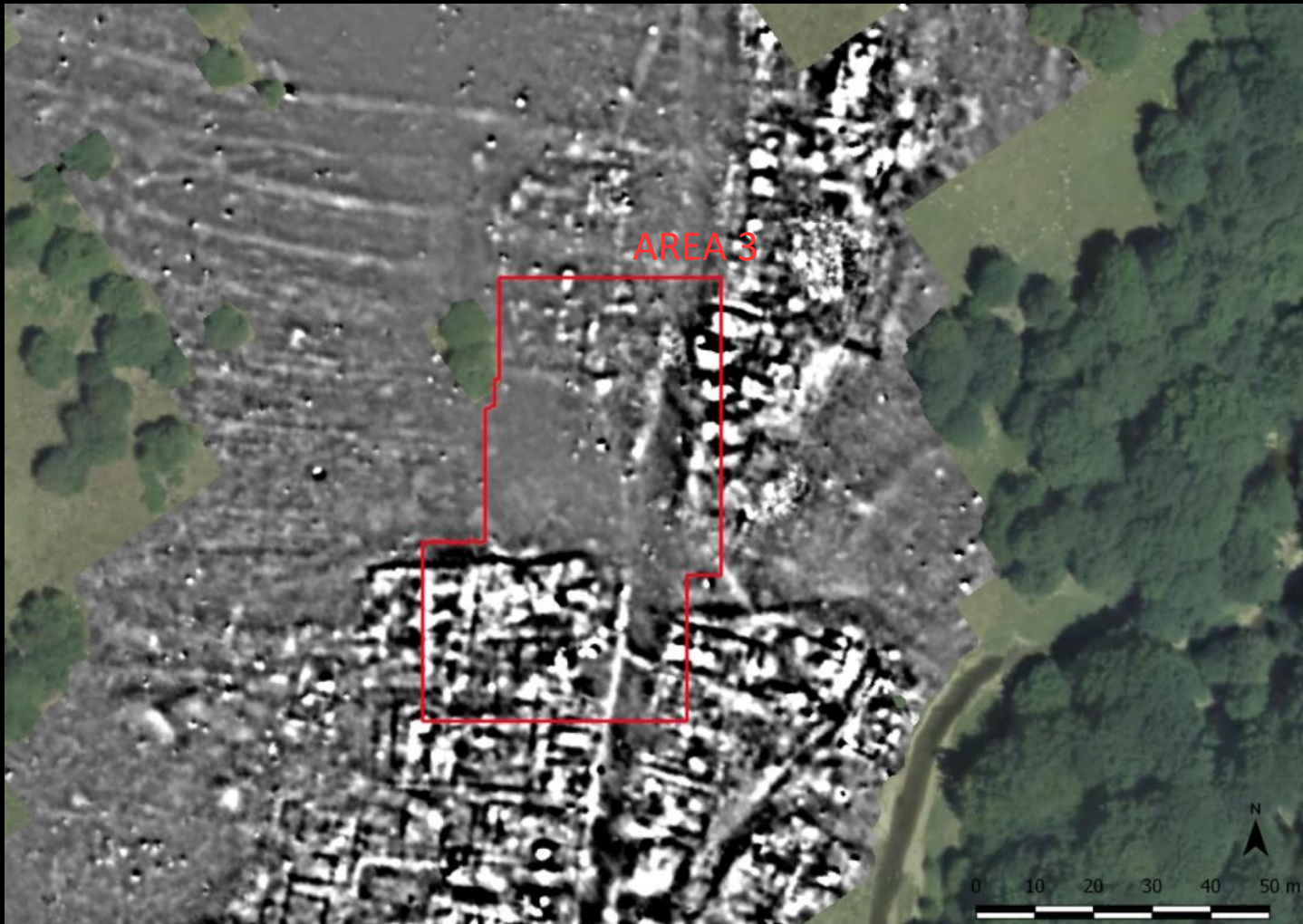
Bartington Grad 601-dual fluxgate gradiometer. Processed data. -7n (black) /+7nT (white)
