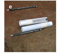
(e) For protection of the core two half PVC tubes and a PVC cylinder (or a cylindrical plastic box) are put together with masking tape to form a support. It is important that there is a slot, as seen on the picture, where later the mark on the core can be drawn.
