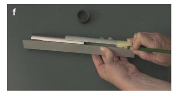
(f) The tube with the core is then removed and inserted in the support. The orientation mark from the tube is thereafter transferred with a pencil along the angular slat to tape on the support.
