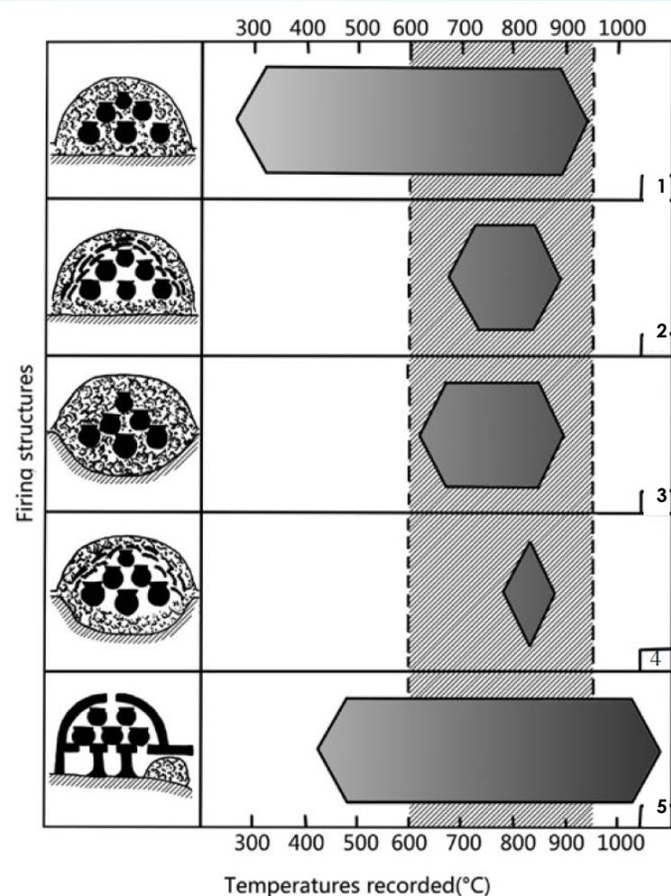
**Figure 3** Temperature ranges for the five kinds of firing.
