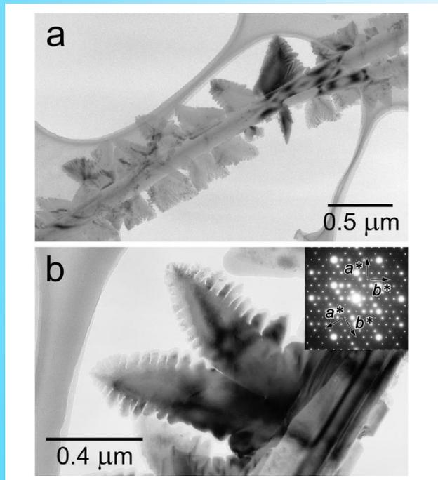
TEM images of  $\epsilon$ -Fe<sub>2</sub>O<sub>3</sub> crystals from ceramic sample from Japan (Kusano et al., Chem. Mater. 2008, 20, 151–156)
