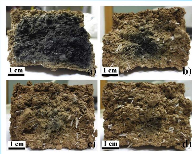
Experimental mud bricks fired at 600°C for time durations:
