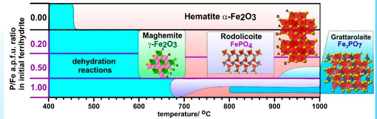
Schematic presentation of temperature ranges of phase stability during thermal transformations of P-doped ferrihydrite (source: Pieczara et al., 2020, *Materials*)
